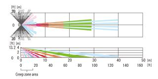
The detection angle of the creep zone can be adjusted  $\pm 135^\circ$  horizontally as shown in gray.
